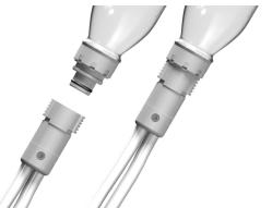
Connect the hose to the FLO Connector. There will be an audible snap when it is locked in place.
